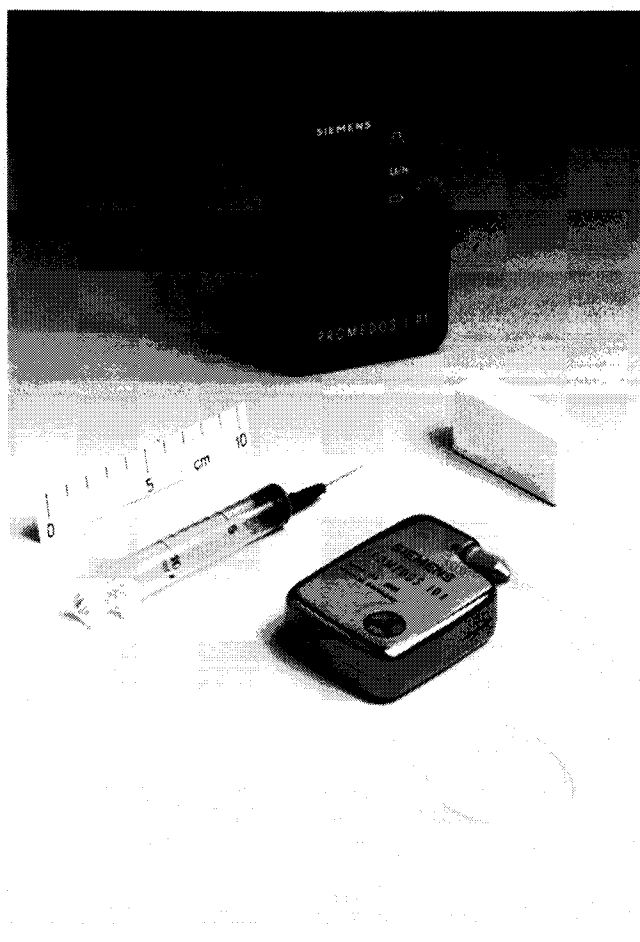
Fig. 4 Implantable insulin pump that operates according to the roller pump principle, type PROMEDOS I 1 from Siemens Company with externally portable programming unit in the background.
